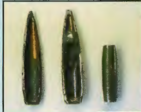
(larger photo) Soviet 5.45mm (right) and 5.56mm U.S. round (left) for comparison. (inset) Sectioned view of the Soviet 5.45mm bullet.
