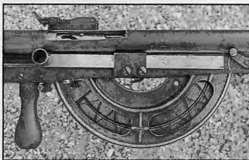
Without doubt, the Fusil Mitrailleur (Machine Rifle) Mle 1915 CSRG, more commonly known as the "Chauchat," was the worst machine gun ever fielded. (below) Cut away on the right side, presumably so that the operator could easily identify the number of rounds remaining, these openings provided ingress for the mud and debris of the battlefield. Worse, the magazines were made of insubstantial sheet metal and all too easily damaged.
