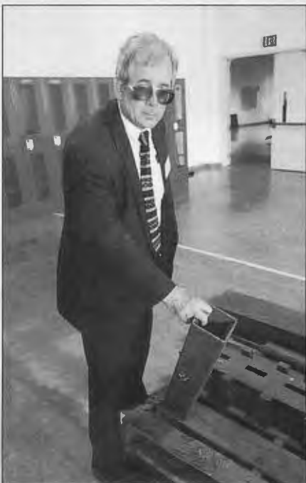
Many components unique to WMDs are similar in appearance to dual-use or garden-variety industrial components. Here Dr. Bill Cliff shows "sharp-edge" graphite components for nuclear reactors. Designed to hold nuclear fuel cells, they may look like components to an electro-winning cell, but are unique to nuclear applications, and suspect.
