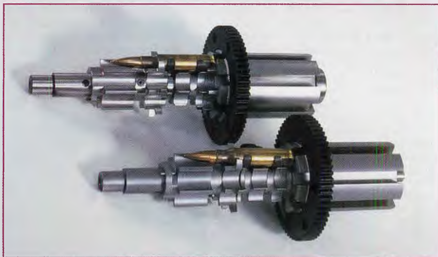
(above) The use of tracer ammunition permits the M134 gunner to walk rounds onto the target and deletes the requirement for a sight system. (right) Dillon stripper, push rod guide and drive gear (top) mounted on feeder/delinker main shaft, compared to original assembly. Numerous improvements enhanced reliability to a significant extent.
