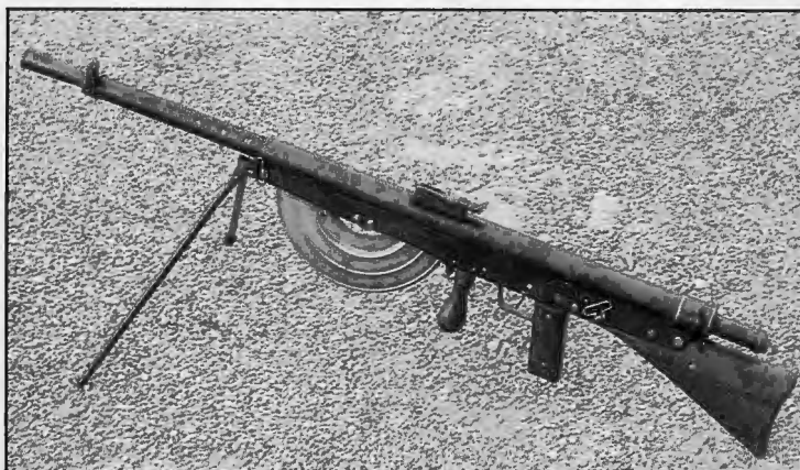
Without doubt, the Fusil Mitrailleur (Machine Rifle) Mle 1915 CSRG, more commonly known as the "Chauchat," was the worst machine gun ever fielded. (below) Cut away on the right side, presumably so that the operator could easily identify the number of rounds remaining, these openings provided ingress for the mud and debris of the battlefield. Worse, the magazines were made of insubstantial sheet metal and all too easily damaged.
