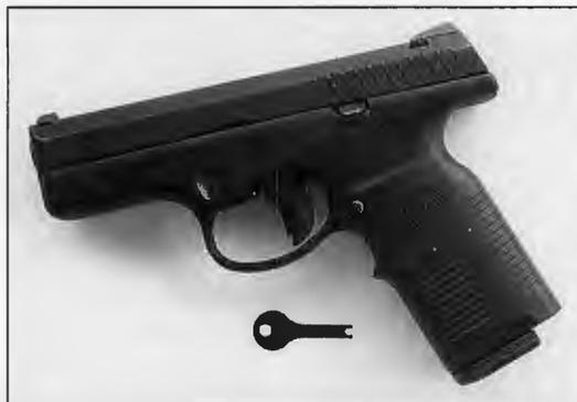
Steyr M9 polymer-framed pistol is chambered for the 9mm Parabellum cartridge. Shown is the key provided with the commercial version for the limited-access lock.
