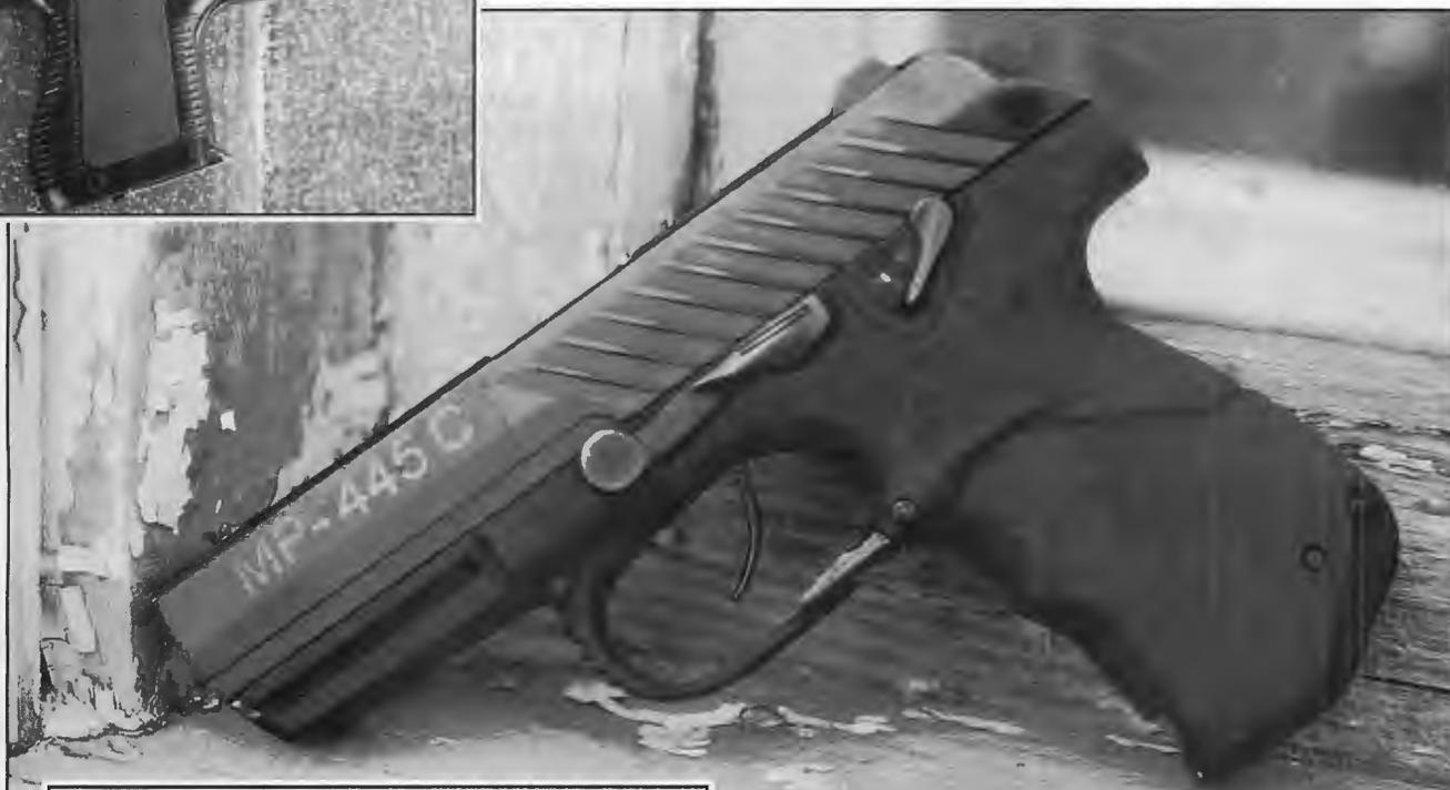
(above) The MP-445C VARYAG (the Norman warrior who founded the Russian state) is a 9mm Parabellum pistol with a polymer frame. Short-recoil, locked-breech operation, with locking in the ejection port, this pistol features double/single-action trigger system, an exposed hammer and a 13-round magazine.
