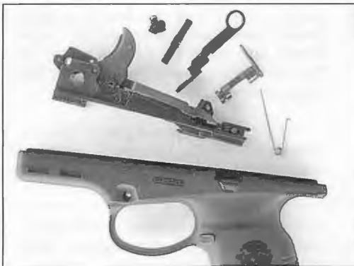
(left) The modular slide guide, which can be easily removed from the frame, contains the trigger assembly, manual safety and slide release lever. (below) Steyr M40 pistol, fieldstripped.
