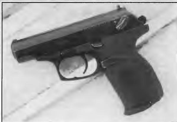
(above, inset) The new Russian Makarov with a polymer frame. Chambered for the 9mm Makarov round, it has a 12-round magazine. The only design change was the addition of a disassembly lever. (right) The MP-446 VIKING is a 9mm Parabellum pistol with a polymer frame and fully adjustable rear sights. It has an exposed hammer and is the "expert" version of the GRACH.
