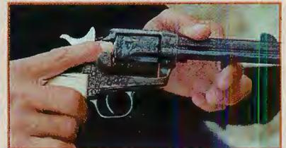
(left) Loading by feel: With the trigger finger firmly up against the base of the cartridge, press rearward on the ejector rod. If it goes only a short distance, as shown, you have encountered a live round. Rotate the cylinder to the next chamber. (right) Again, with the trigger finger firmly up against the base of the cartridge, press rearward once more on the ejector rod. If it goes fully rearward, as shown, you have encountered an empty case. Eject the case and load a live round.
