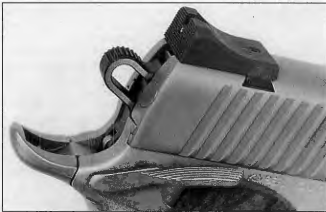
(above) Ambidextrous safety, a Custom Shop feature, allows the operator to fire with the support hand only. (right) Author installed Heinie Slant Pro
