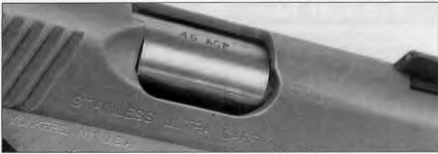
The ejection port has been lowered and flared to enhance ejection reliability and protect empty cases from denting. (right) Author's battery of working Kimbers, from top to bottom: Custom Classic with Alternative Force Block, Stainless Steel Gold Match, Compact Custom and new Stainless Steel Ultra Carry.
