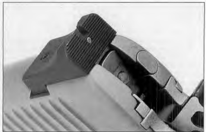
sights with tritium inserts as they are designed for one-handed clearance drills and provide an excellent sight picture for firing under stress.
