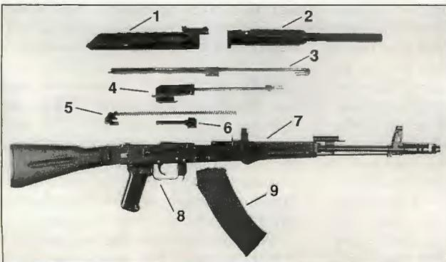
Main parts and assemblies of the AL-7: 1 — top cover with rear sight, 2 — gas tube with steel cover, 3 — upper rail with gas piston, synchronizing sprocket and return spring, 4 — bolt carrier with gas piston, 5 — return mechanism of bolt carrier, 6 — bolt, 7 — barrel with receiver, stock and hand-guard, 8 — trigger and trigger mechanism, 9 — magazine.
