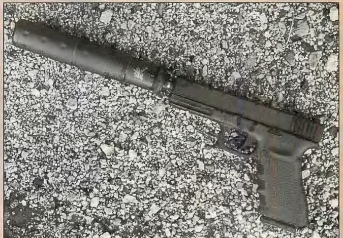
obtained with the suppressor in place to within 2 inches of the unsuppressed shot group. With the suppressor firmly tightened on the barrel, an orientation mark on the suppressor body should be more or less upper-dead-center when commencing to index the suppressor to the sights with live-fire. Indexing the suppressor to change the point of impact takes only a few minutes.
