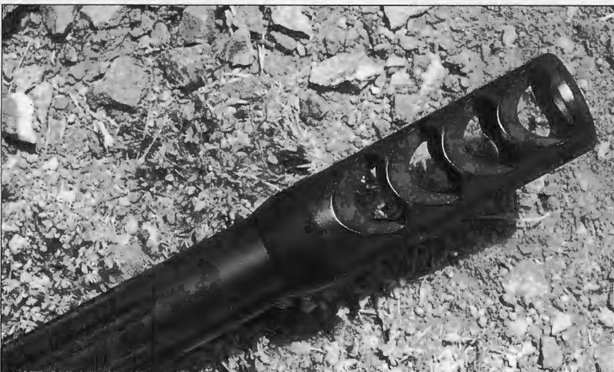
2,000-plus hours in a 5% salt spray. It possesses some self-lubricating properties as well. The Roguard process involves preparation of the base metal and then phosphating. Afterwards, the Roguard is sprayed on and then baked to cure at low temperature.
