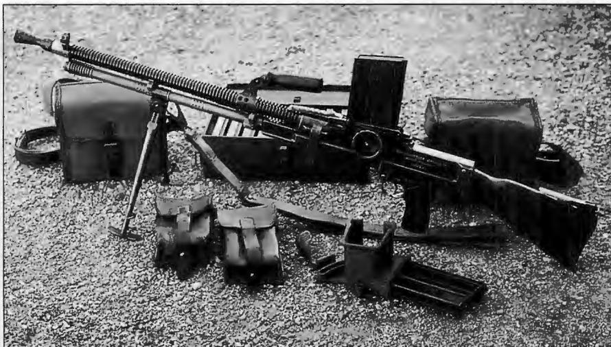
ZBvz26 with an assortment of two-magazine leather pouches for harness carry, steel magazine chest, heavy canvas magazine boxes and magazine loader. (left) These 40-round ZBvz26 magazines were manufactured in the 1930s at Zbrojovka Brno for anti-aircraft use. ZBvz26 gunner's wallet (below) with cleaning equipment, oil bottles, broken case extractor, spare flash hider and an elaborate combination tool.
