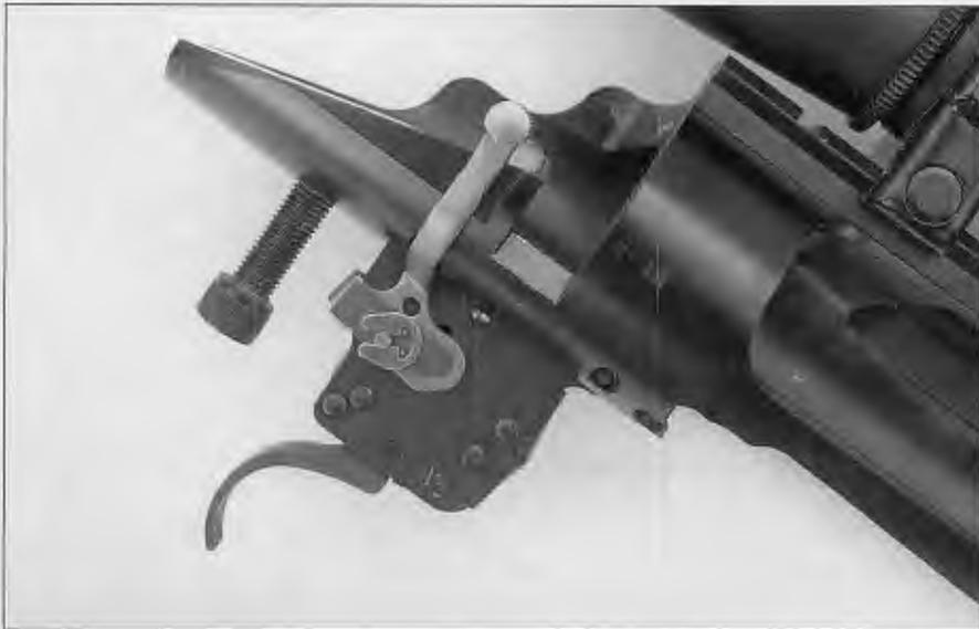
(above) Robar RC50 .50 caliber rifle uses a Remington 700 trigger and safety mechanism. (below) RC50 muzzle brake is smaller and more efficient than any currently on the market.
