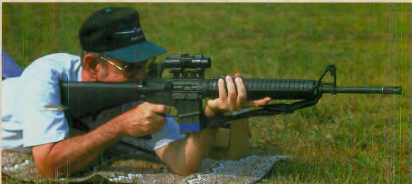
SSK AR-15 T-SOB installs red dot sight in place of suitcase handle on AR-15 upper receiver. Original iron sights remain in place. If bat-
