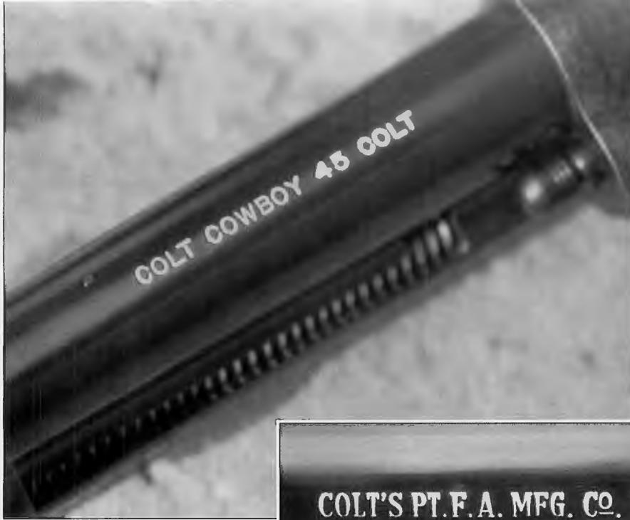
(above) Roll mark on left side of Colt Cowboy barrel. (right) Roll mark on top of Colt Cowboy barrel is that of third-generation Model 1873 SAA revolver.
