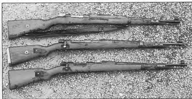
Earlier Yugoslav Mausers include, top to bottom: M24/52 with a straight bolt handle, followed by two K98k types
