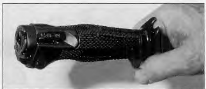
Safety lever located in butt of knife (muzzle of gun) exposes a red dot when in firing position.
