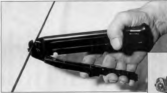
An operator can cut wire or steel rods of 5 mm, or (inset) electrical wires to 400 volts (note: never cut wire suspected of being energized, two at a time.)
