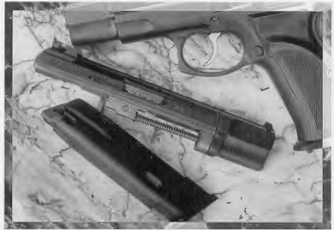
Kadet .22 LR conversion kit is blowback-operated; provides the same weight as a 9mm CZ75B and comes with one 10-round magazine.
