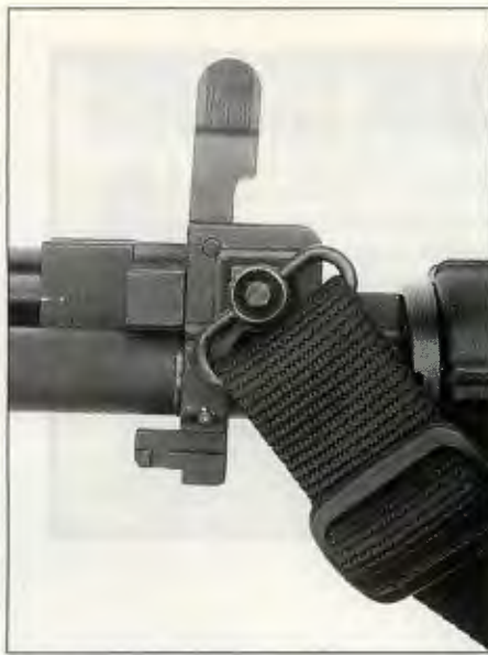
G.G. & G. fold-down front sight system for the M16/AR-15 series. Note Uncle Mike's QD sling swivel and bayonet lug. (right) G.G. & G. fold-down front sight system in the down position. This permits use of optical equipment without an annoying and distracting ghost image of the front sight assembly.
