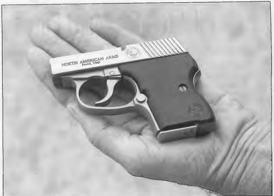
NAA Guardian represents the latest trend in minuscule pocket pistols: a .32 ACP chambering in a .25 ACP envelope. (below) Right-side view; note slide release button on the frame directly under the cocking serrations and used for disassembly.
