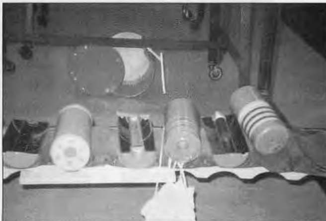
U.S. chem/bio bomblets (left to right): BLU 21/B45 biological bomblet; BLU 20/B BZ bomblet; BLU 19/B23 GB bomblet.
