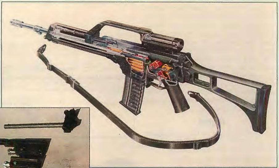
Cutaway view of G36 hints at the AR-18 ancestry of the bolt and gas system; (inset) G36 bolt, carrier and operating spring (top) compared to those of the original AR-18.
