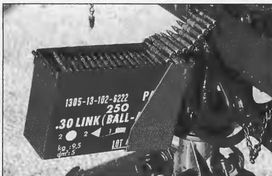
**Kent Lomont's bracket permits use of the now more common .30-caliber ammo cans without the latching mechanism on the M1917A1 tripod.**
