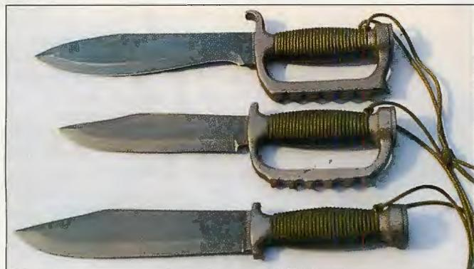
the tang and wrapped with paracord, and have a steel endcap for pounding. They come with a heavy leather scabbard.
