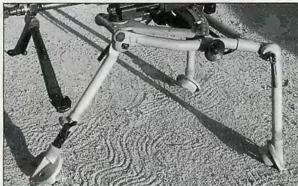
Israeli FN MAG 58 tripod, constructed mostly of titanium and aluminum. Note telescoping front leg. Tripod would never be deployed in combat with the legs in this position.
