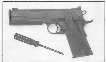
the thumb safety, which, after many thousands of rounds, was sometimes dropping the hammer. The front strap was checkered to 20 LPI and hex-head grip screws were installed for cosmetic reasons. A pair of Kim Ahrends cocobolo tactical grips were also installed.
