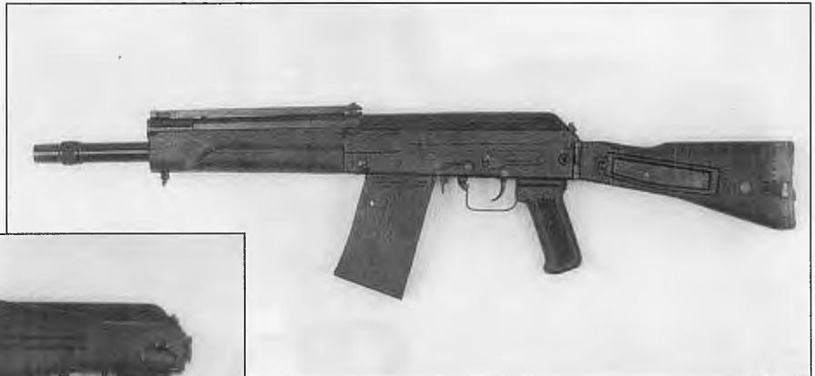
(above) Left side of Saiga-12K shotgun: knob on rear of receiver serves to deactivate the weapon when buttstock is folded. (inset) shows buttstock folded. (below) Saiga-12K semi-automatic shotgun, fieldstripped. Simple, robust Kalashnikov design adapted well. Note enlarged bolt head and strengthened bolt carrier.
