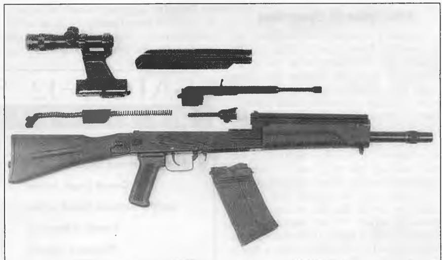
Capacity of the Saiga-12’s black, fiber-reinforced polyamide magazines is five rounds “standard” or seven rounds on special order. Experimentally, the factory had made welded sheet-metal 10-round magazines, but Izhmash has carried out numerous tests to determine the optimal size for such a magazine. The best compromise between the desire to increase capacity (only natural from a tactical point of view) and practical experience, is five to seven rounds.
