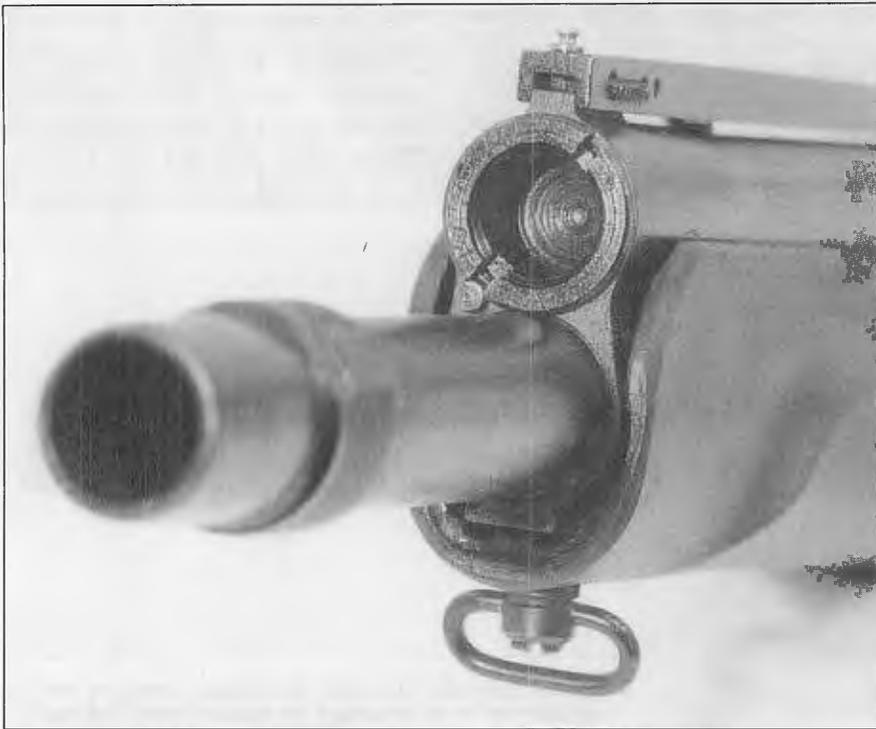
Business end of the Saiga-12K shotgun is *all* business: Note choke muzzle attachment, gas regulator, sling swivel, black synthetic handguard, front-sight brass bead on the serrated rib. By turning wheel, sight is adjustable for elevation.
