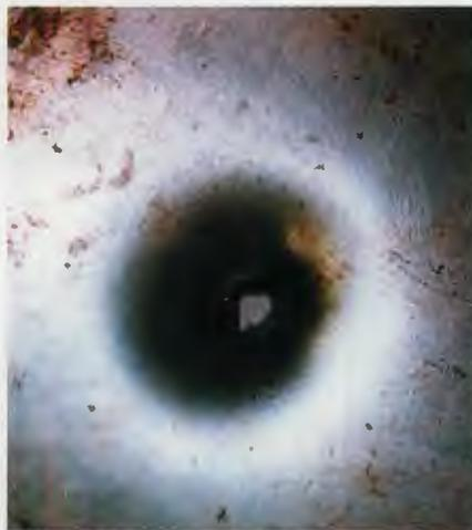
Polev sub-caliber 511.5-grain lead slug fired at a distance of 55 yards blew through 0.08-inch steel plate.
