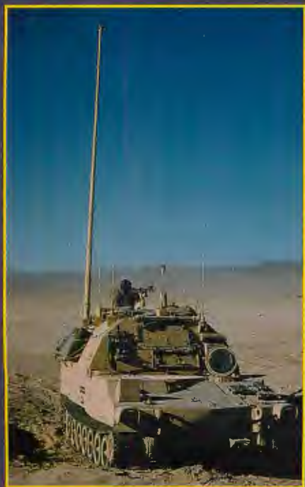
(above) The M113 is the work horse for all mechanized units. A strip of buttons near the front of the vehicle detects bursts of laser energy during practice battles, shutting all weapons down if the vehicle is "hit" by weaponry the computer deems capable of destroying it in real life. (left) Built by United Defense, this Fire Direction Center Vehicle (FDCV) is designed to receive information from the Support Team (FIST) vehicle and direct fire based on that information and other data coming in from commanders in the field. Also known as the Field Artillery Operations Center Vehicle, the unit provides ballistic protection against direct and indirect fire.
