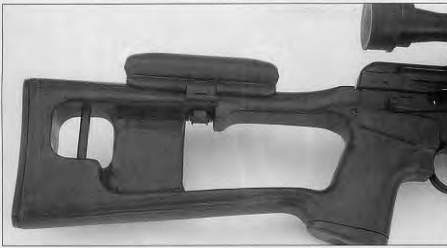
NORINCO .308 SVD is equipped with the usual skeletonized, wood-laminate buttstock, with a leather padded cheekpiece that can be removed.
