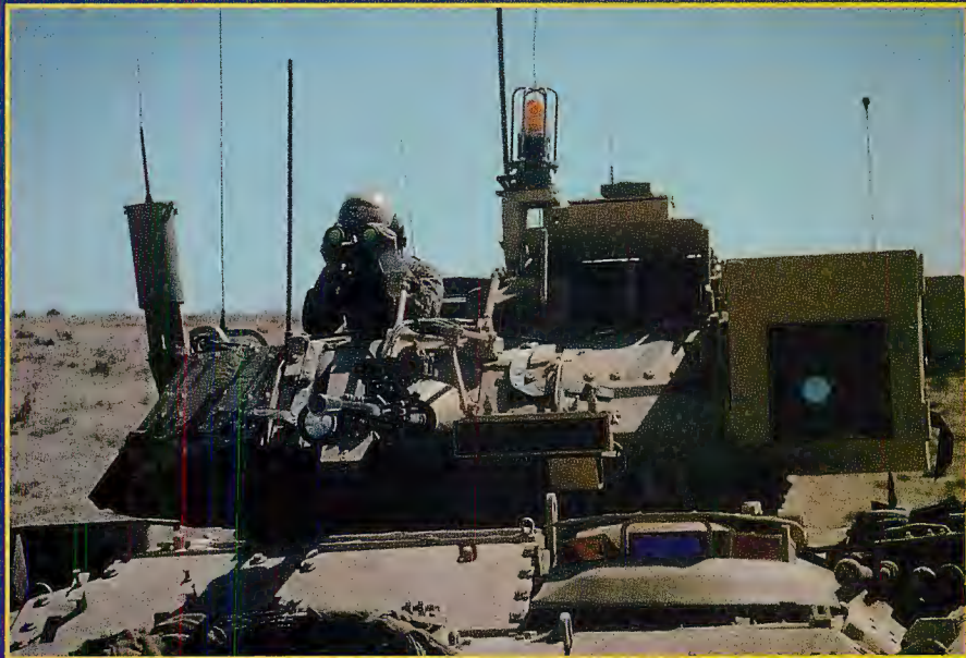
(above and left) The Bradley Fire Support Team (FIST) Vehicle serves as the eyes of the artillery. It can plan, coordinate and direct artillery fire in timely and accurate fashion. These FISTs are each equipped with a 25 mm Bushmaster Chain Gun. (below) This Israeli-built Hunter Short Range Unmanned Aerial Vehicle is remote-controlled and used at the NTC for battlefield observation. It takes real-time video, giving commanders a bird's eye view of the fight. It can loiter in the air for eight hours, at a ceiling of 1,500 feet.
