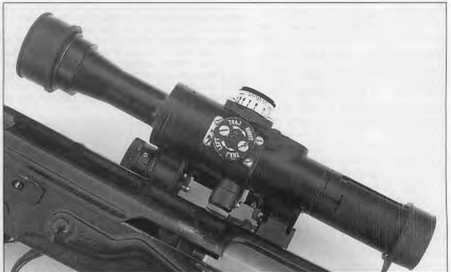
Scope found on NORINCO .308 SVD is a copy of the Russian four-power PSO-1, but with markings in English. It is under-powered and the reticle pattern is too busy for long range shooting under the stress of combat.
