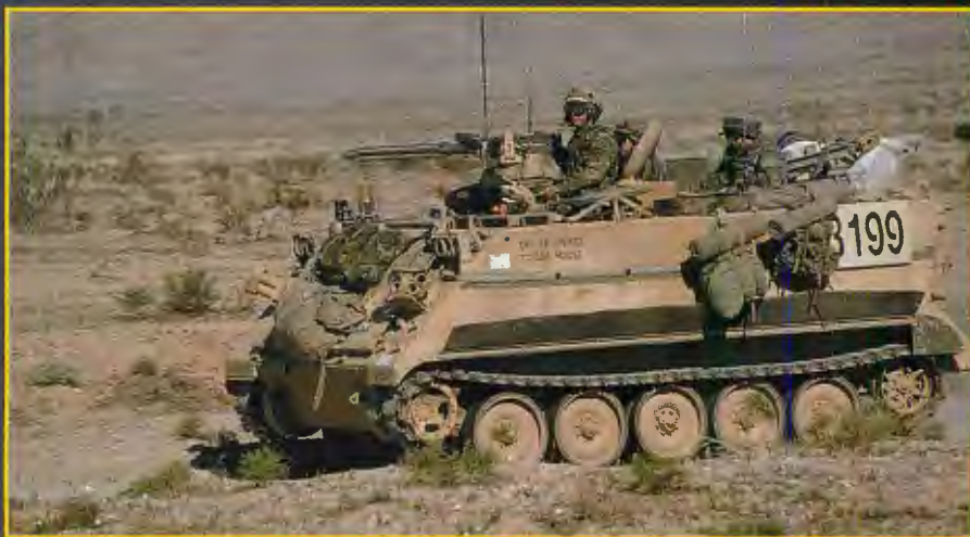
(above) The M113 is the work horse for all mechanized units. A strip of buttons near the front of the vehicle detects bursts of laser energy during practice battles, shutting all weapons down if the vehicle is "hit" by weaponry the computer deems capable of destroying it in real life. (left) Built by United Defense, this Fire Direction Center Vehicle (FDCV) is designed to receive information from the Support Team (FIST) vehicle and direct fire based on that information and other data coming in from commanders in the field. Also known as the Field Artillery Operations Center Vehicle, the unit provides ballistic protection against direct and indirect fire.
