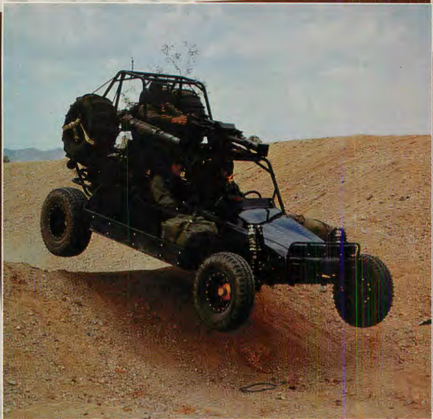
(opposite) Airborne! (Well, almost). The Chenoweth Desert Patrol Vehicle (DPV) avec M60E3 GPMG, AT-4 rocket launcher and Mk19 MOD 0 40mm machine gun. (above) Not the Baja "One-Thou," but the Chenoweth FAV working out in California's Mojave. (below) The Chenoweth Advanced Light Strike Vehicle (ALSV). Quite simply, "The fastest and most agile military vehicle in the world."
