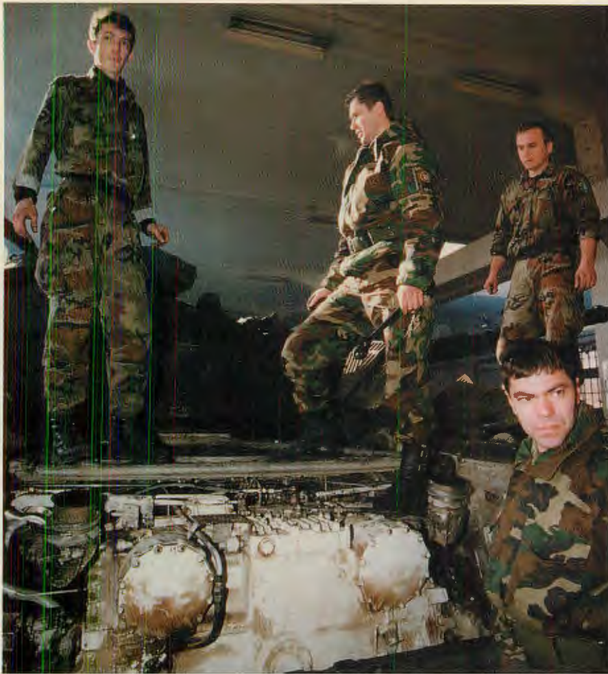
(left) As a team, Bosnian and Croat soldiers service an M60A3 tank at Hadzici motor pool. Many had prior training in Turkey on M60A3. (above) MPRI instructor at Hadzici motor pool shows HVO crew how to use tanker's bar and come along to close belly escape hatch (which had probably been opened to clean tank from top down, inside and out).
