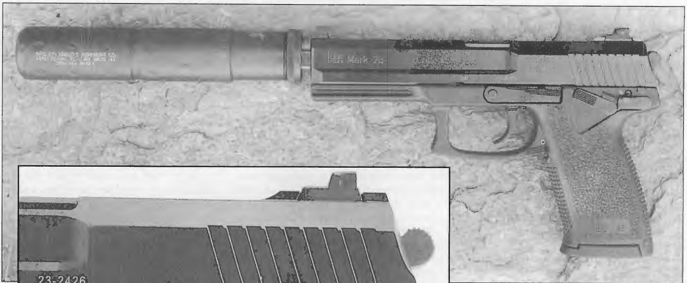
(above) Overall length of the Mark 23/MK23 MOD O, with the sound suppressor attached, is 16.58 inches. The weight with a loaded 12-round magazine is 4.23 pounds. (inset) All of the Mark 23/MK23 MOD O controls are close at hand. From left to right: slide-release lever, decocking lever and ambidextrous manual safety lever.
