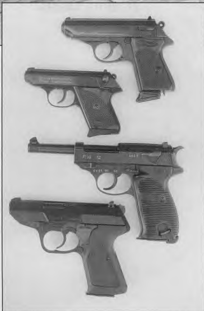
(above) The P99's polymer frame provides exceptional strength and durability. This locked-breech, short-recoil-operated pistol has a double-action trigger system with a unique decocking bar on the slide. (right) Walther's line of famous handguns have included (top to bottom): the PPK ( Polizei Pistole Kriminal ), TPH .22 LR/.25 ACP pocket pistol, World War II-era P.38 and its post-war derivative, the P5 Compact.
