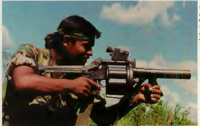
FOE uses Armson OEG collimating-type sight to find range of target for South African Mechem MGL 40mm grenade launcher.
