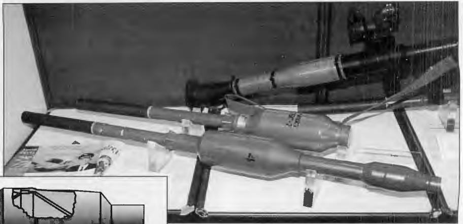
The TBG-7 thermobaric round (top) and PG-7V round comprise leading-edge upgrades. The TBG-7's FAE is an effective weapon on buildings and bunkers; the PG-7V two-stage round is intended to defeat new developments such as reactive armor.
