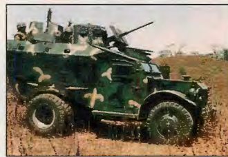
Two types of Salvadoran warwagons that saw heavy use in ops against FMLN rebels: German-made UR-416 APC (left) with .50-caliber heavy machine gun, and locally developed Cashuat , here in gun-carrier variant with one M2HB forward and an M60 on each side.
