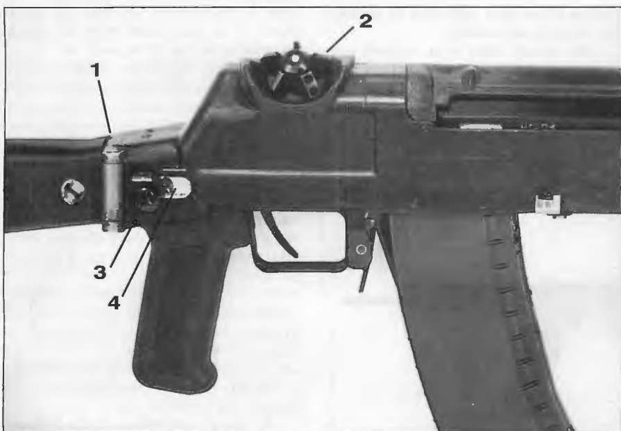
(above) Closeup of AN-94 shows 1) hinge for folding butt stock, 2) rotary asterisk-type diopter rear sight, 3) butt stock lock-release button, and 4) trigger-mechanism release lever. (right) Underside of weapon shows 1) magazine latch (the magazine attaches at an angle to give extra space for the return spring), 2) safety shift lever (position "II" for safe, position "O" for fire), 3) fire-mode selector, 4) cleaning rod.
