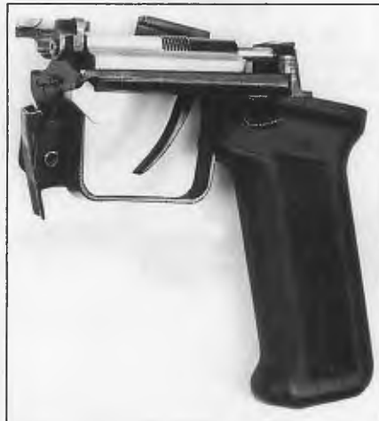
Pistol grip integrated with trigger mechanism, safety lever, selector and magazine latch.
