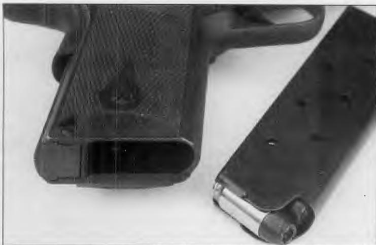
(left) The magazine-well is beveled to assist changing magazines. The magazine holds eight rounds and has McCormick's famous Shooting Star two-piece follower and follower spring. (right) There are deeply cut cocking serrations both fore and aft on the slide. Since this pistol is equipped
