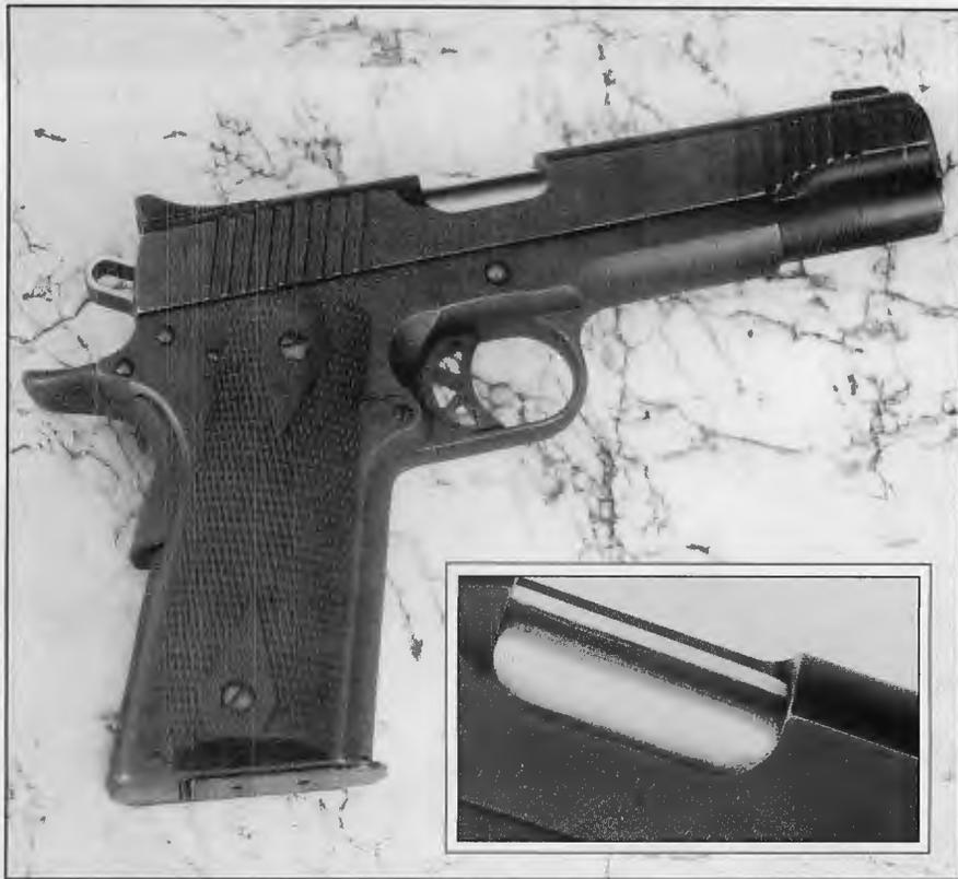
The ejection port has been lowered and flared in the now standard "custom" manner to enhance ejection reliability and protect empty cases from denting.
