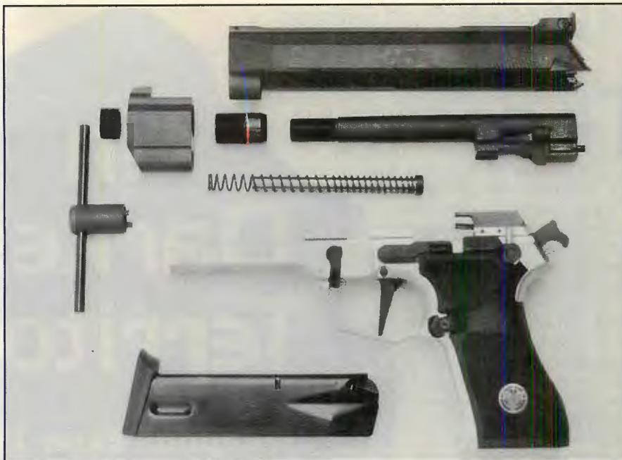
The front of the SP1 Target Model's barrel has an adjustable tapered lock nut that interfaces with the front of the slide. Using the differential screw-thread principle, the purpose is to remove all play between the slide and barrel. A wrench and instructions are supplied.
