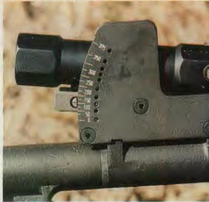
**The MGL Mark I is equipped with an Armson OEG collimating-type sight which provides a single vertical red bar. It requires binocular vision on the part of the operator, who aims with both eyes open and sees the aiming bar superimposed on the target**
