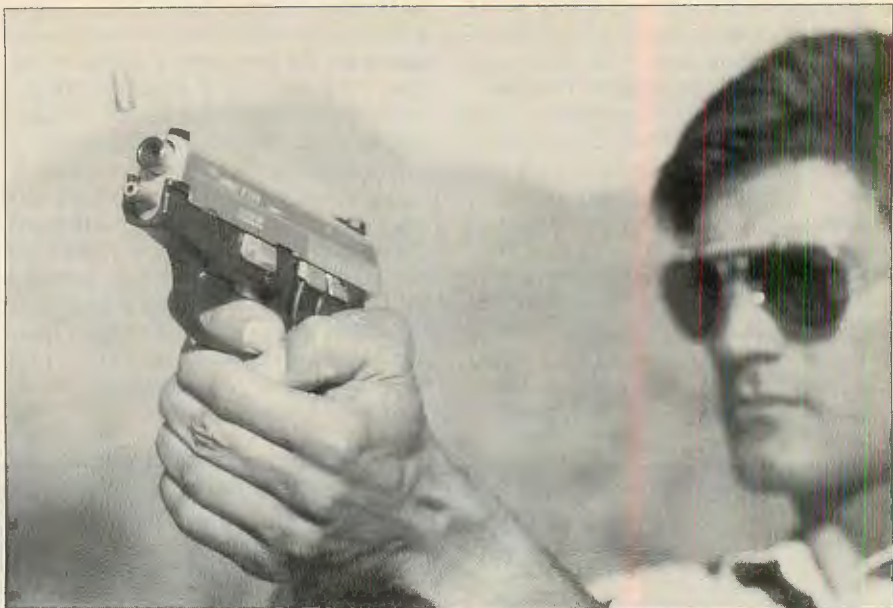
With a black-anodized, aluminum-alloy frame and weighing only 27.5 ounces, empty, the compact SIG-Sauer P239, chambered for the 9mm Parabellum cartridge, exhibits very little perceived recoil.
