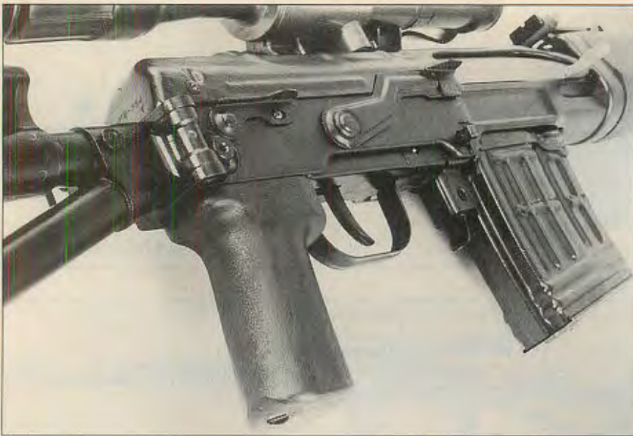
The SVDS buttstock hinge, buttstock lock knob, top (bolt) cover locking lever, and safety selector lever.
