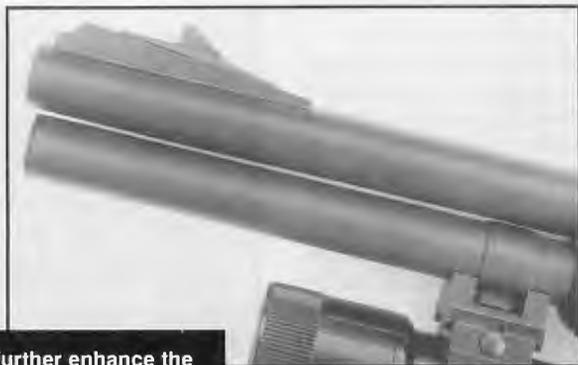
**To further enhance the accuracy potential, the front barrel band of the Model 1894 was completely removed to free-float the barrel.**
