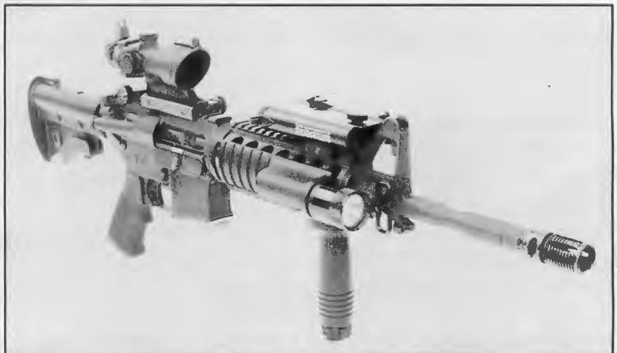
M4A1 carbine with a KAC flip-up rear sight and Trijicon ACOG optical sight attached to the upper receiver's rail. The KAC RIS is fitted with an infrared laser aiming module, flashlight and vertical foregrip. Note KAC flash hider attached to the muzzle which permits installation of their quick-detachable sound suppressor.
