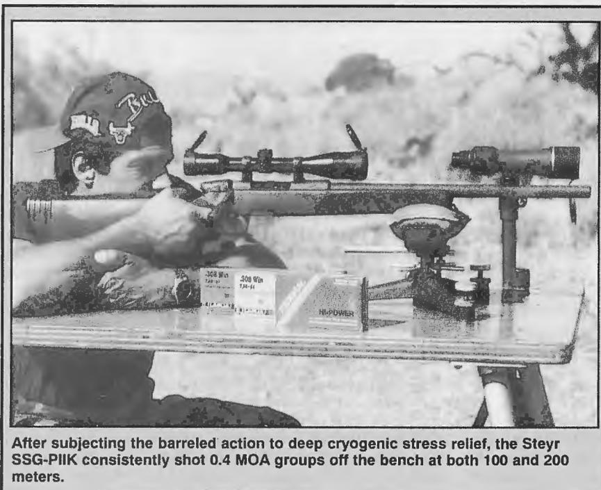
After subjecting the barreled action to deep cryogenic stress relief, the Steyr SSG-PIIK consistently shot 0.4 MOA groups off the bench at both 100 and 200 meters.
