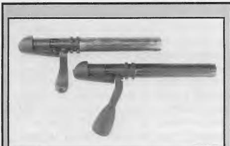
Both the original Steyr SSG 69 bolt (top) and that of the SSG-PIIK (bottom) are identical except that the SSG 69 bolt had a so-called "butterknife" bolt handle while those of the Police series have large knob-type bolt handles.
