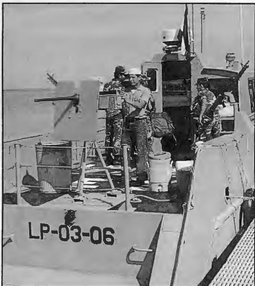
A .50-caliber M2 HB Browning and two 7.62mm M60 general-purpose machine guns provide aft firepower on Salvadoran naval patrol boat used in territorial waters where bullets might fly over fishing disputes or drug interdiction.
