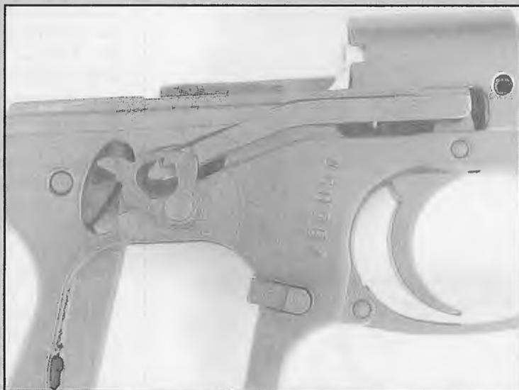
**In the double-action mode, a pull on the trigger will draw the trigger bar forward. This rotates the sear forward on its axis pin, causing the hammer-cocking bent to be drawn forward and up, thus raising the automatic safety tumbler out of the hammer's path and rotating the hammer on its axis pin to compress the hammer spring. As the sear slips out of the cocking bent, the hammer falls.**
