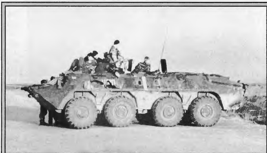
Roadblock in Chechnya: Russian soldiers atop a BTR-70 armored personnel carrier (APC) monitor traffic. This class of amphibious APC commonly is armed with one 14.5mm and one 7.62x54R machine gun, and carries a crew of two plus eight infantrymen.
