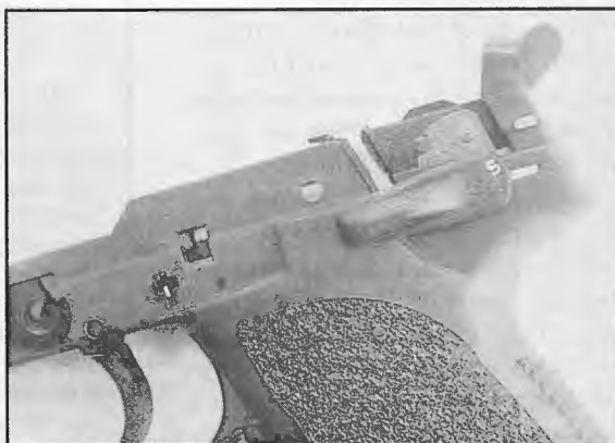
All of the various fire modes and control functions available for the USP series are determined by a notched detent plate inside the frame, to which the safety lever, if present, is attached.
