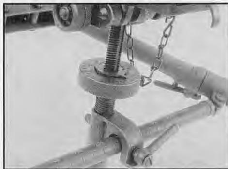
The M2/M122 tripod's traversing bar has an engraved scale to assist in measuring or establishing horizontal angles. The elevating handwheel assembly has a mil click device built into it. Note that the 50-mil scale engraved on the upper surface of the handwheel is divided into 5-mil major graduations and 1-mil subdivisions.
