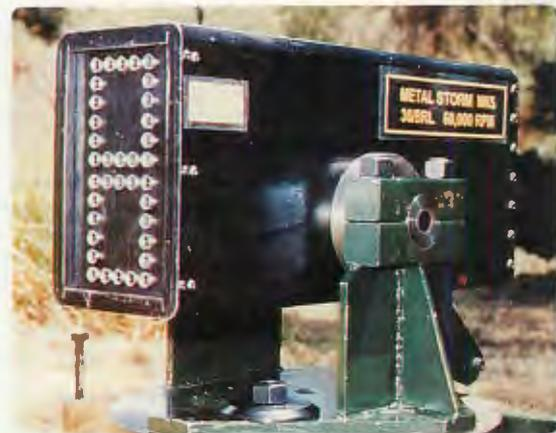
This Mk5 prototype of Metal Storm's 36-barreled pod system might be the shape of vehicle- or helicopter-mounted suppressive-fire weapons of the future. The prototype was considerably overbuilt for safety reasons. It comprises three-barreled sections, all of which have delivered 45-round bursts at a rate of 135,000 rounds per minute.
