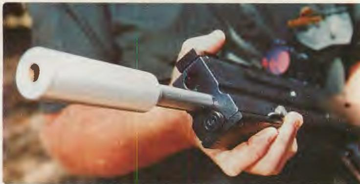
The 15-shot weapon, configured for hand-held use, is remarkably compact. Because it has no heavy, reciprocating bolt knocked rearward with each discharge, the test weapon is surprisingly easy to control during rapid fire.
