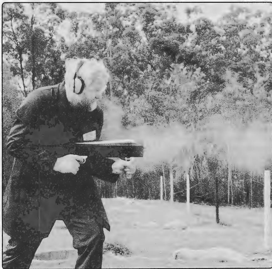
In an early test, gunsmith Graham Bugden fires a three-round burst from the nine-barreled prototype. Since there are no moving parts to reciprocate nor any cartridge cases to eject, the rounds can be fired virtually in a continuous stream, just as fast as bore pressure drops to a safe level after each shot. The maximum theoretical rate approximates 45,000 rounds per minute, per barrel, assuming uninterrupted reloading.
