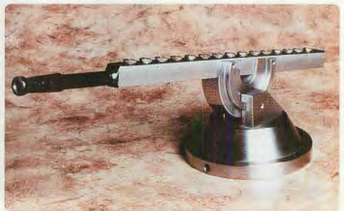
With its casing removed, the single-barreled prototype's 15 external priming ports, in which ball powder is loaded, are visible along the top of the barrel. Note the difference in effective barrel length between the first and last rounds of the payload; this can affect a projectile's ballistic performance.
