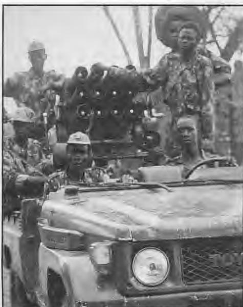
The SPLA's mobile artillery: a multiple-rocket launcher that was captured from the Sudanese army and mounted on a light truck.
