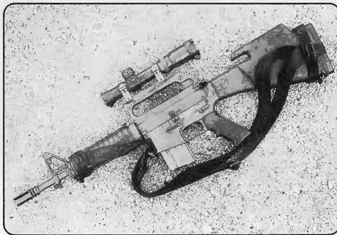
Author entered Gunsite’s #223 Tactical Carbine course thinking he had a really hot setup. The Vortex flash hider, Giles sling, fixed buttstock and 20-round magazines proved to be ideal. But, among other deficiencies, the Delta H-BAR cheekpiece interferes with the cocking motion when the retracting handle is pulled rapidly rearward. Furthermore, the scope was too high above the bore for close-range shooting.
