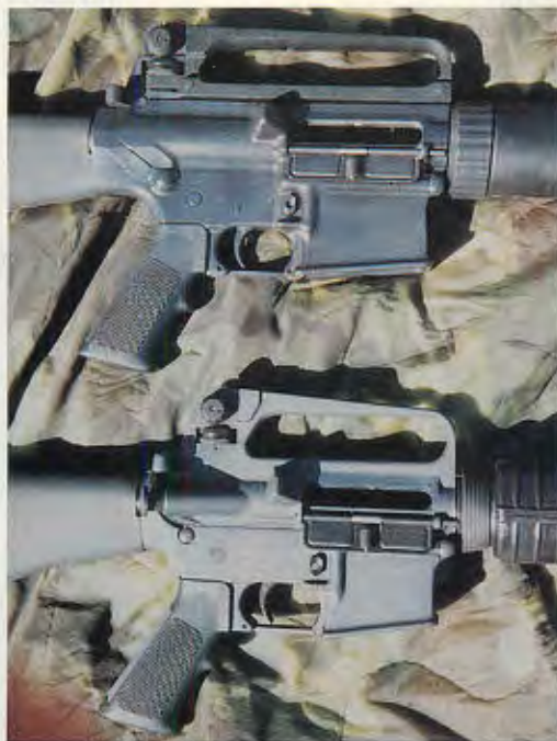
With new tooling, the ArmaLite AR-10A2 (top) was able to incorporate such M16-series improvements as the case deflector, belled magazine well and protected magazine release button — plus refinements such as detachable sight bases that reveal a Picatinny rail.
