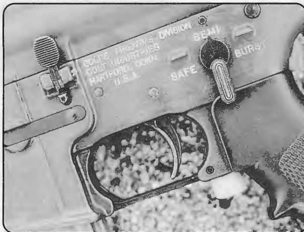
The gap in back of the hinge that permits the bottom of the M16's trigger to be rotated down for winter firing with gloves can pinch the second finger of the firing hand. A temporary fix is to insert a foam ear plug into the gap.
