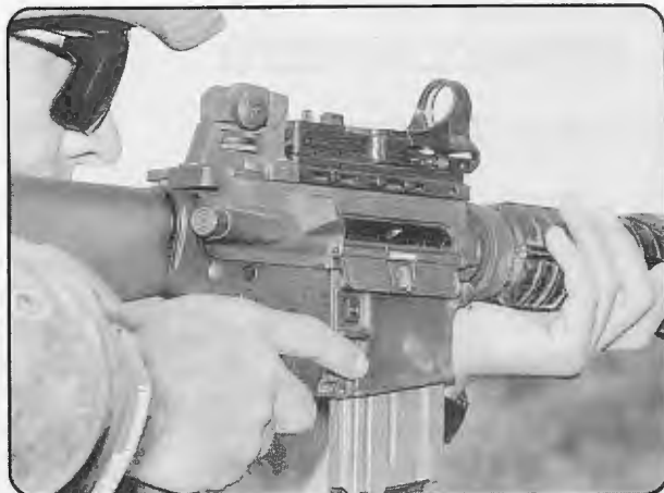
The C-More sight's red dot is projected onto a single lens by a small LED projector in the base. If and when the small opening from which the beam of light projects clogs with mud, the red dot is gone and the sight becomes useless. Furthermore the lens, although protected by a sturdy steel ring, sits above the sight's body and would all too easily be damaged in the harsh environment of the battlefield.
