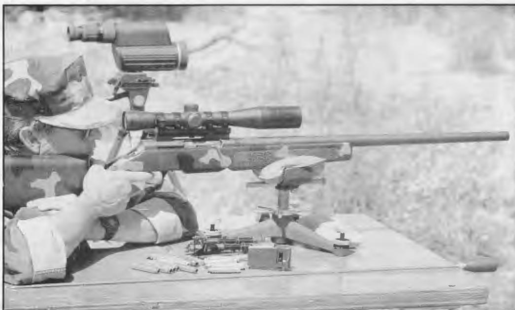
**Super Match Interdiction Rifle provides accuracy potential that compares favorably with the best bolt-action sniper weapon systems and surprisingly mild perceived recoil for a caliber .300 Winchester Magnum rifle.**
