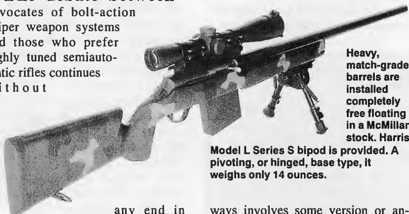
Heavy, match-grade barrels are installed completely free floating in a McMillan stock. Harris
