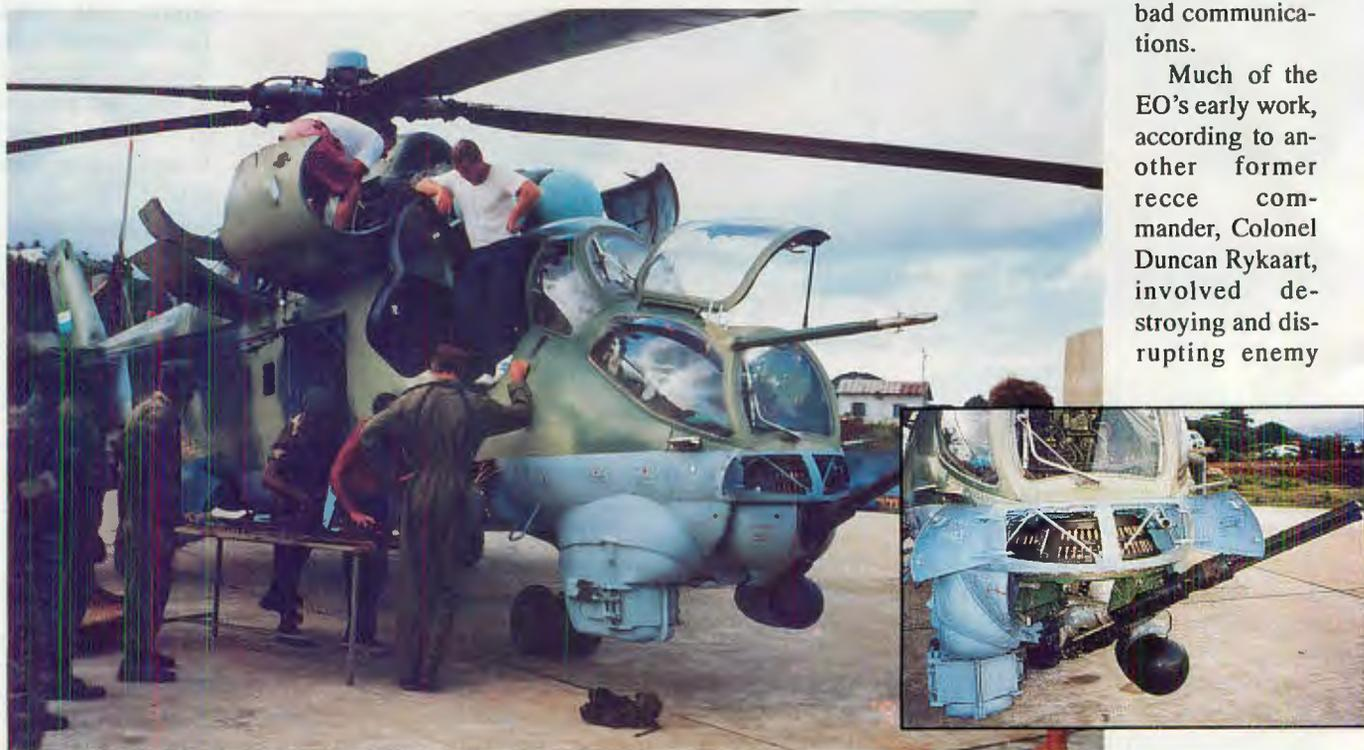
In EO actions in Sierra Leone, Russian Mi-24 "Hind" attack choppers have proved to be tough and deadly, mounting a variety of ordnance including (inset) a four-barreled 12.7 mm machine gun and 1,300 rounds of ammo.
