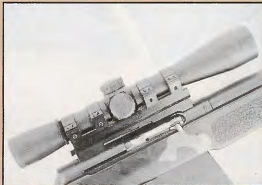
**Leupold Mark 4 M3-10X scope attached to Super Match Interdiction Rifle by means of the sophisticated Arms Tech Ltd. Omega mount, which is machined to extremely close tolerances to permit repeated removal and reinstallation of optical sights without loss of zero.**
