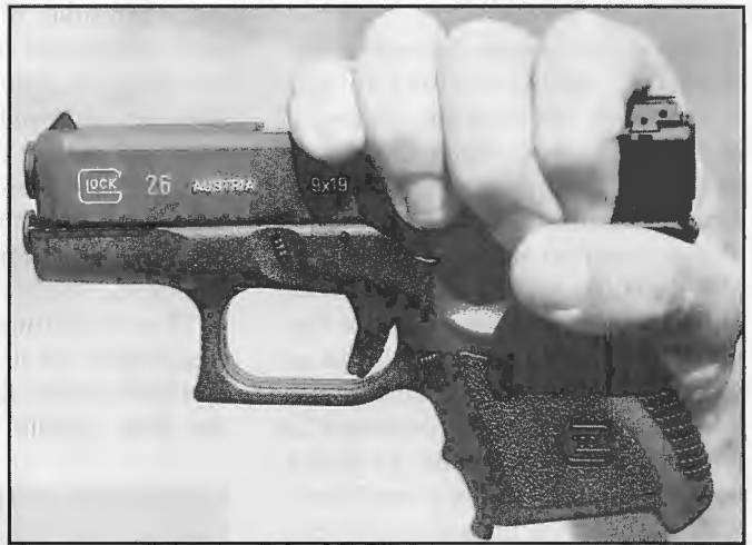
The first step in separating the slide from the frame is to retract the slide about an 1/8-inch in the manner shown.
