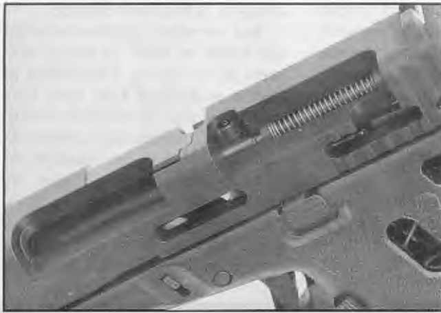
Unique factory cutaway shows the Glock's spring-loaded firing-pin safety blocking the striker's forward movement.
