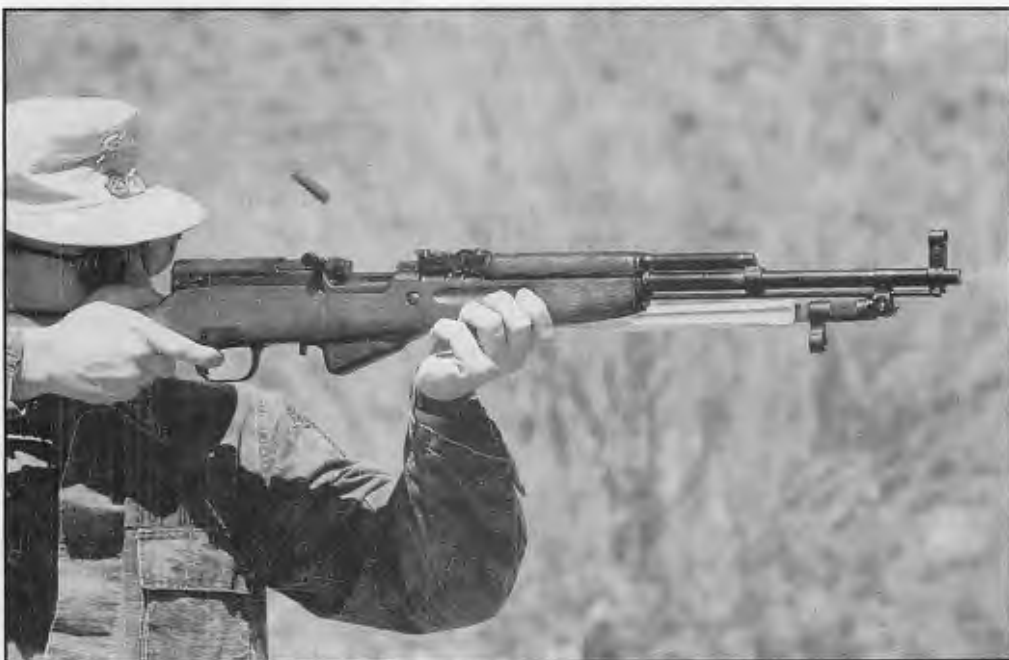
As a consequence of the SKS carbine's weight — heavy by today's standards — and the intermediate-size cartridge for which it is chambered, perceived recoil and muzzle jump are inconsequential.
