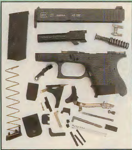
Glock Model 27 caliber .40 S&W pistol, completely disassembled.
