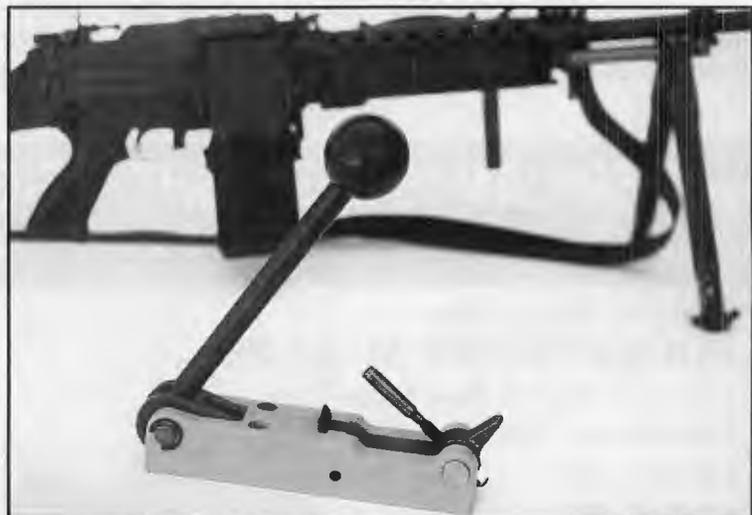
Those who intend to reload using surplus military cases, which almost always have primers that are staked or ring-crimped in place, are well-advised to obtain the Dillon Super Swage 600, a tool designed specifically to remove the crimp and permit a new primer to be properly seated in the pocket.
