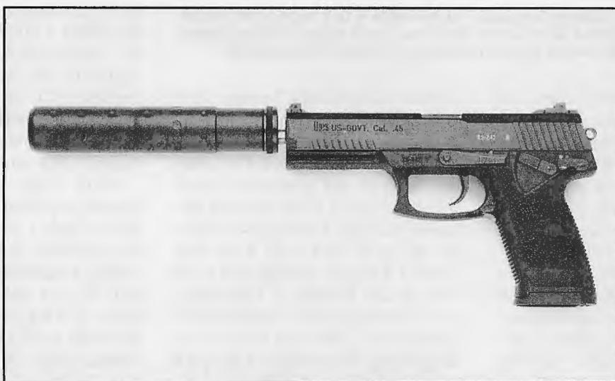
**Heckler & Koch's Phase II Offensive Handgun differs from their original Phase I entry. The slide lock has been removed and the safety lever is 0.15-inch wider to permit the operator to obtain a better purchase with gloves. The hammer has been changed to a hollow spur, which will deform if impacted upon during a drop test and thus prevent a primer indent.**
