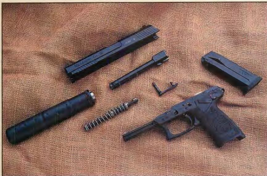
**H&K SOCOM Phase II pistol fieldstripped. The handgun is to a large extent based upon their USP and operates by means of short-recoil with breech locking, based on a linkless modified Browning system (ejection port barrel-locking block).**
