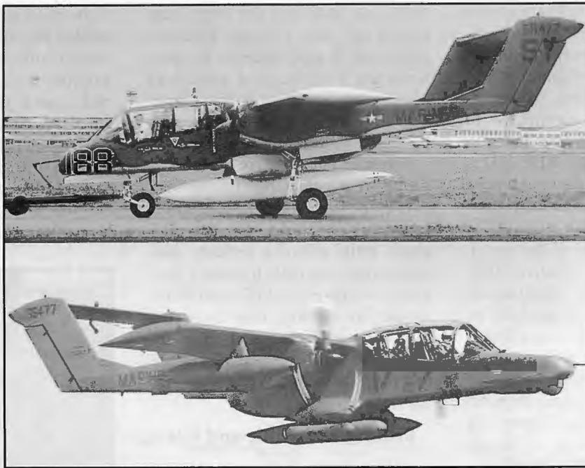
Agile, capable, field-maintainable, the OV-10 proved itself an excellent close-support combat craft from Vietnam to the Gulf War. Top photo of "155477" shows original OV-10A configuration at roll-out during 1969 Paris air show. Bottom photo is of same plane modified to OV-10D specs, over Ohio in 1980. Photos: Norman Taylor Collection
