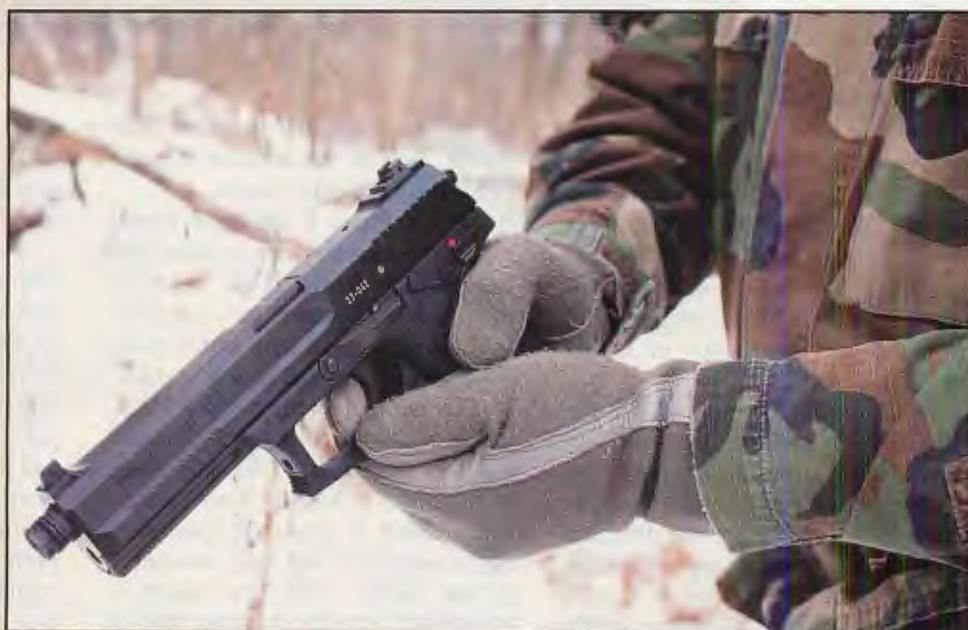
**The weapon is designed to fire a minimum of 30,000 rounds of +P ammunition (5,000 with the suppressor in place), without any major parts failure or replacement. The slide and frame were designed for a minimum of 60,000 rounds.**
