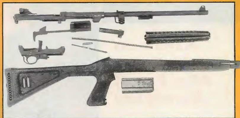
MAG-1 .45 Winchester Magnum Carbine, fieldstripped.
