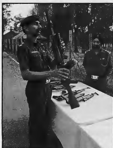
Smuggled weapons captured from insurgents included this one-man assault team based on an East-German MPIKM that features sound suppressor, BG-15 type 40mm grenade launcher, high capacity RPK-style drum magazine.
