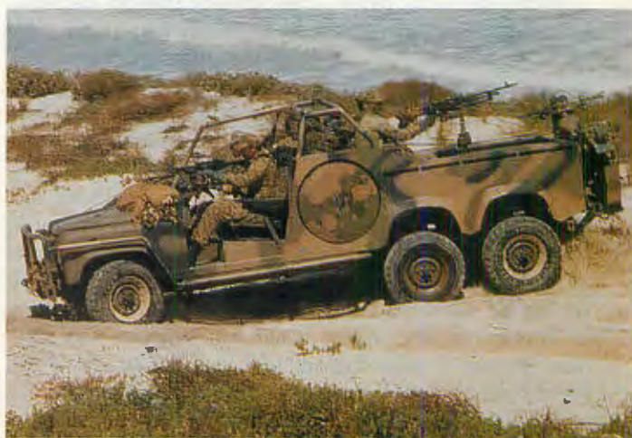
SAS variant of Hotspur One Fifty carries 7.62x51mm NATO L7A2 GPMG (General Purpose Machine Gun), F89 MiniMI machine gun and a dirt bike. Unique combination of equipment, training and personnel qualify SAS as world-class elite unit.
