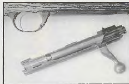
Ruger M-77 Mark II bolt handle is integral with the one-piece bolt body that has dual-opposed forward locking lugs and a long one-piece, Mauser-type extractor attached to the bolt body by a collar. The extractor does not rotate with the bolt.
