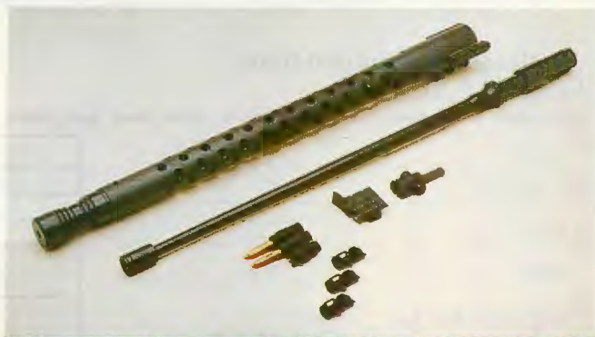
GA1 .50 caliber conversion kit consists of barrel jacket assembly, .50 caliber barrel with integral piston at muzzle, 12.7x99mm bolt head, feed ramp and plastic link inserts.
