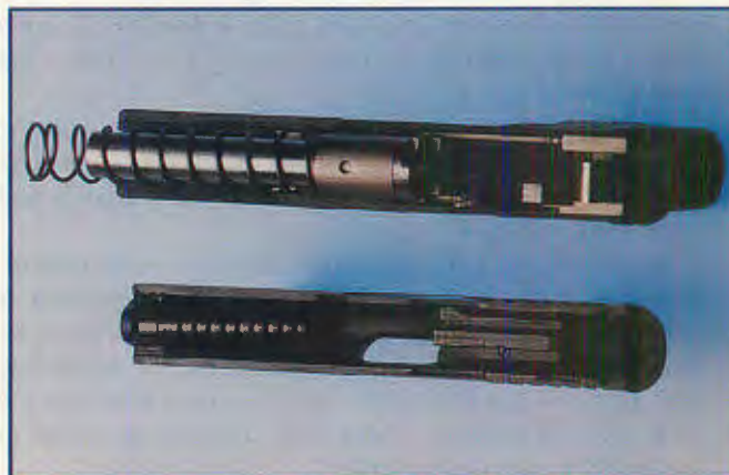
Top: While the CP1's barrel does not move during the recoil cycle, the barrel and gas block to which it is pinned can easily be removed from the frame. Bottom: CP1 gas piston is hinged and attached to the front of the slide. Photo: courtesy LIW
