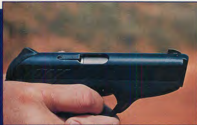
CP1 front sight is adjustable for windage. Fixed, open square-notch rear sight is part of the slide casting. Photo: Peter G. Kokalis
