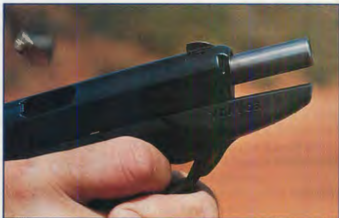
CP1 exhibits somewhat less muzzle jump than would be expected from a 24-ounce pistol chambered for the 9mm Parabellum cartridge. Photo: Peter G. Kokalis
