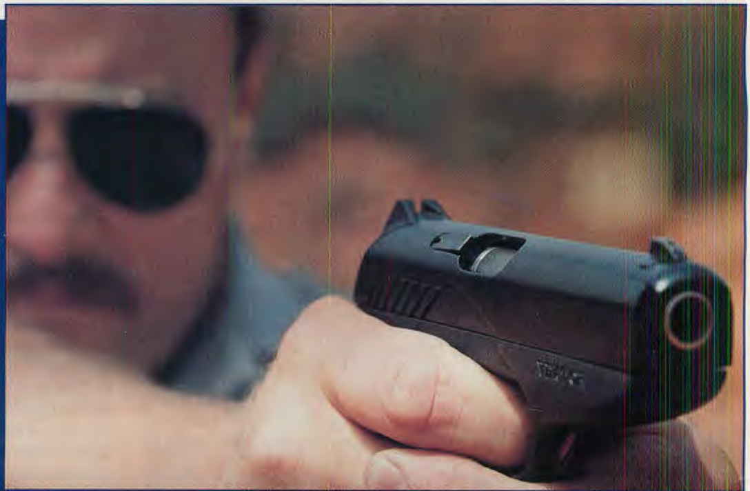
South African CP1 is not only eye-appealing, but exhibits human engineering at its small arms zenith. Note location of manual safety in the front end portion of the trigger guard. Photo: Peter G. Kokalis
