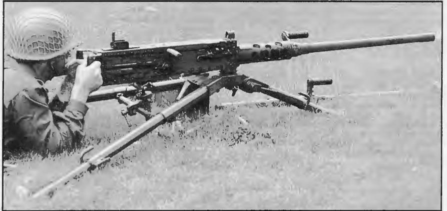
Still the world's very best heavy machine gun, John Browning's .50-caliber M2 Heavy Barrel, fired here from the sturdy M3 tripod, has been brought to the highest possible levels of performance by important modifications introduced by FN Herstal. Photo: Peter G. Kokalis
