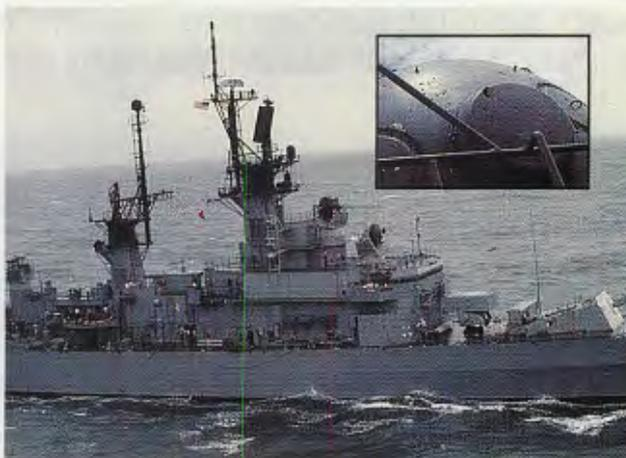
Starboard side of USS Worden after she absorbed two Shrike anti-radar missiles fired by a "friendly" jinked-out jet jockey returning from a mission over Haiphong. Inset: Worden's fire control radars took hundreds of shrapnel hits — protecting all but one of the 50 men in CIC during the errant attack.
