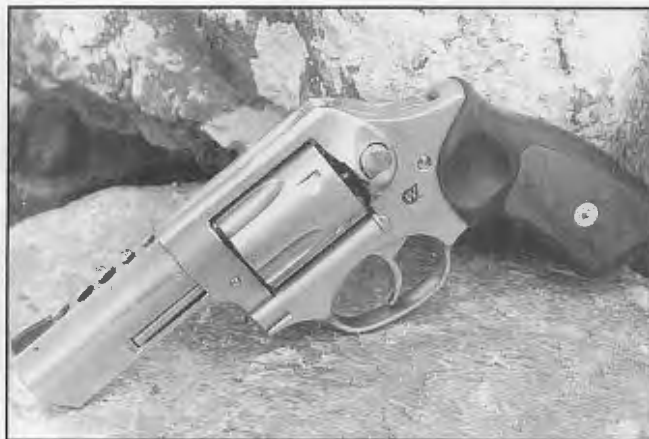
Ruger SP101 .38 Special with 3-inch barrel. Hybra-ported barrel, bobbed hammer and custom tuning by Weigand Inc.
