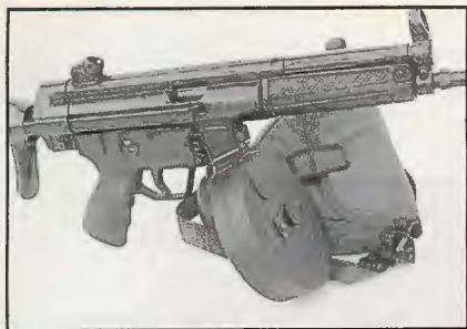
Added firepower for the MP5 series: Modified Russian PPSH-41 drum holds 72 rounds of 9mm Parabellum.
