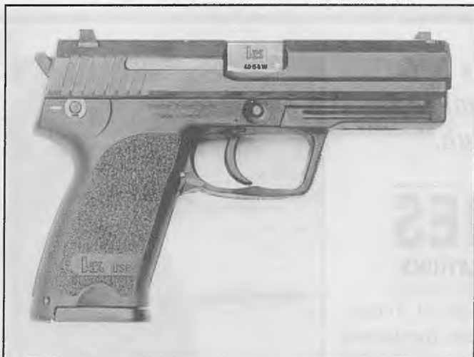
Right-side view of the H&K USP shows the large, rectangular lug over the barrel's chamber that engages the slide's ejection port in the locked position. Note groove on frame forward of trigger guard used for attaching accessories such as a laser sight. "Tear away" notches at the bottom of the grip assist removal of a jammed magazine. Photo: courtesy H&K
