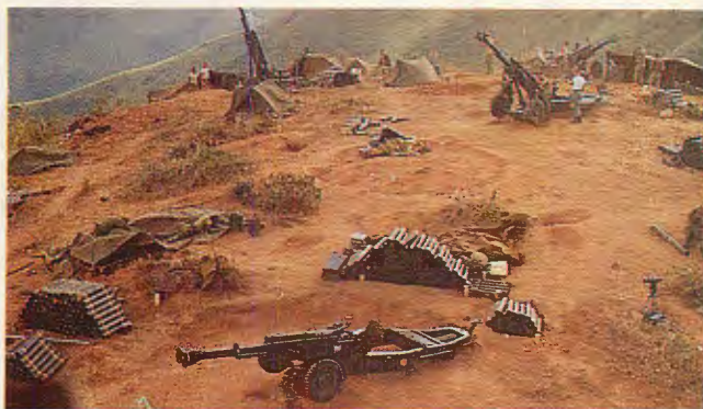
Army firebase in the highlands: Well-sited artillery from these M102 105mm howitzers could provide fire support to a radius of 15 klicks with RAP ammo. We fired more arty, dropped more bombs in Vietnam than in all of WWII ... but it didn't work.
