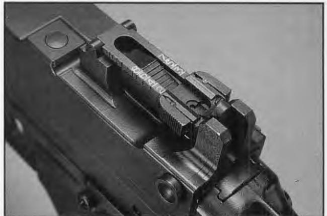
SS-77's folding-leaf rear sight has been taken from the FN MAG 58 and provides a peep aperture in the down position for ranges from 200 to 800 meters.
