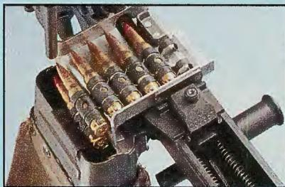
SS-77 feed tray will accept almost any type of belt or links without alteration to the feed mechanism and with no increase in belt drag or reduction in the cyclic rate.
