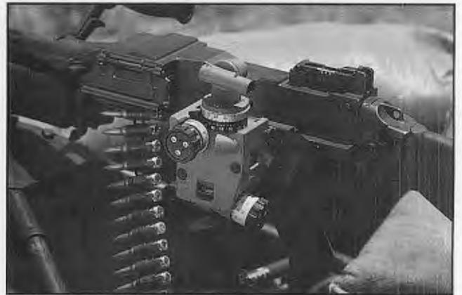
Sophisticated H-019 long-range dial sight can be mounted to the left side of the SS-77 receiver body for indirect fire from defilade along fixed lines.
