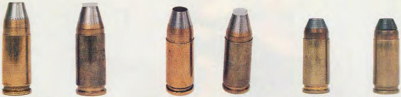
"Cyclone" tubular steel rounds, designed to defeat polyaramid fabric body armor: At left is prototype bullet loaded in Winchester brass for U.S. Army at Aberdeen Proving Ground, Maryland. At right is similar bullet loaded in GEA brass with a high-density polyethylene feeder-tip to facilitate functioning in automatic weapons.
