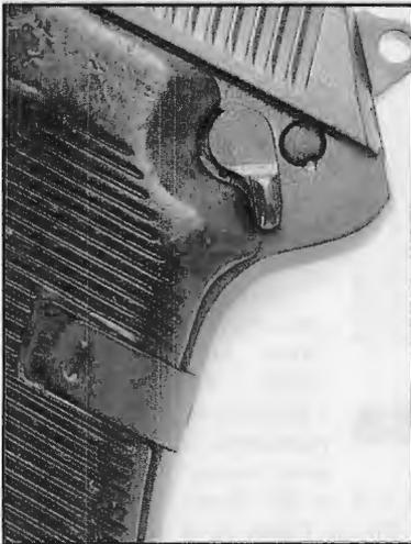
Frame-mounted, three-position safety lever permits the hammer to be safely dropped with a loaded chamber. Horizontally ribbed plastic grip panels are held in place by an odd spring clip.
