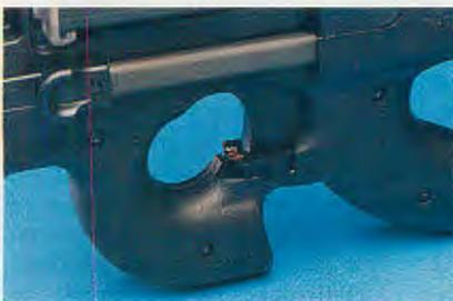
The grip portion of the P90's receiver body has been molded into the configuration of an abbreviated thumbhole stock. The selective-fire dial is directly under the trigger and thus is completely ambidextrous, as are all of the P90's controls.
