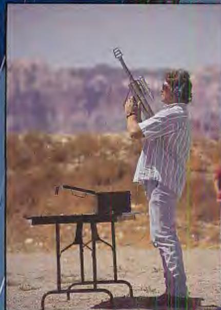
Demonstrator of Maadi-Griffin fired this single-shot .50 caliber pistol with one hand and it didn't break his arm. It did, however, warp the muzzle brake and make a very big hole downrange.
