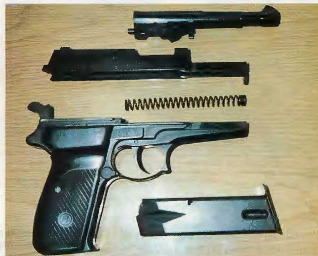
New Croatian PHP MV-15 pistol shows design influence from proven features of Walther, Beretta. Note P.38-type pivoting lock. Photo: Bruno Radovcic
