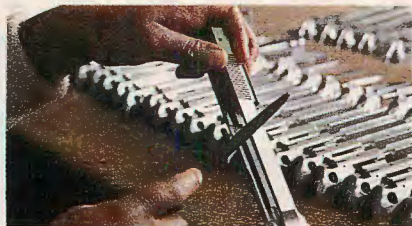
Many steps in the production of a modern firearm must still be done by hand. Z88 slides are deburred with Swiss files.
