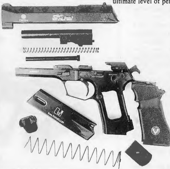
South African SP1 9mm Parabellum double-action service pistol, fieldstripped.
