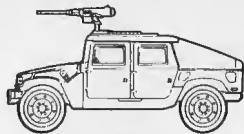
ARMAMENT CARRIER Supplemental Armor W/.50 Cal M2HB MG M1043 W/O W M1044 W/W
