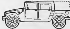
CARGO/TROOP CARRIER Soft Top Enclosure (4-Door Cab, Cargo) M998 W/O W M1038 W/W
