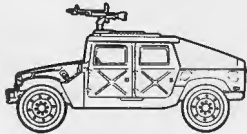
ARMAMENT CARRIER Basic Armor W/7.62mm M60 MG M1025 W/O W M1026 W/W
