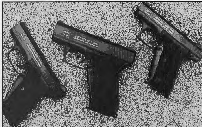
Heckler & Koch's P7-series now includes (left to right): P7M8 — 9mm Parabellum; P7M10 — .40 S&W; and P7K3 available in three chamberings — .380 ACP, .32 ACP and .22 LR.
