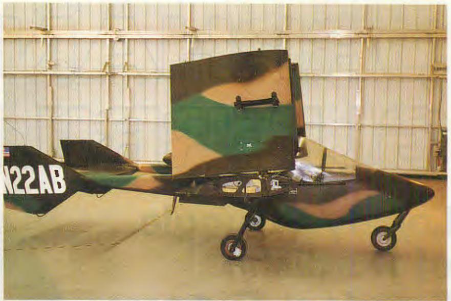
Cheap, simple, rugged Sadler A-22 weighs just 950 pounds, yet delivers 1,000 pounds of ordnance. Wings fold for transport, storage.
