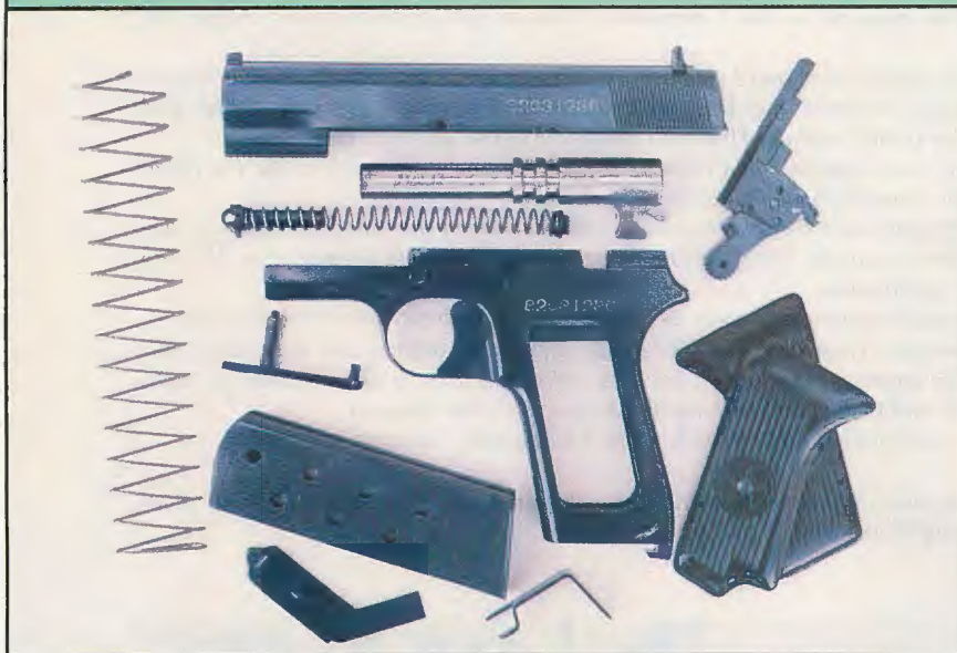
North Korean Type 66 pistol, fieldstripped. Note serial number on left side of frame under the grip panel.
