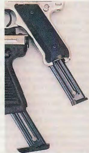
**R**uger 22/45 (left) and Mark II (right) magazines are not interchangeable, as the new 22/45 magazine body's angle with relation to the floorplate had to be changed to accommodate the change in grip angle, while maintaining the same feed angle with regard to the receiver body.
