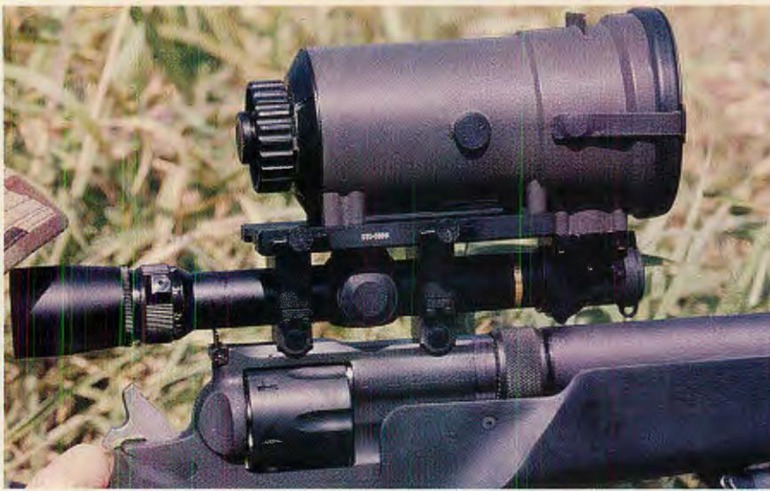
Knight's Revolver Rifle comes equipped with sophisticated optics, including a Leupold VARI-XIII scope and a Simrad KN250 night-vision unit mounted directly over the Leupold. Emergency tritium sights complete the package.
