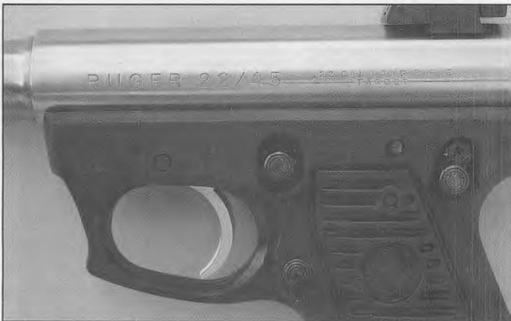
**M**anual safety, magazine catch/release and bolt hold-open release controls on the Ruger 22/45 approximate the location of those on the M1911A1.
