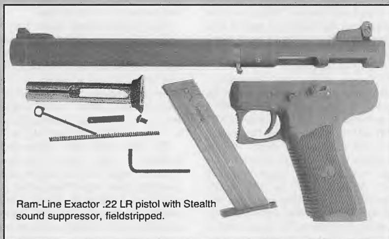
Ram-Line Exactor .22 LR pistol with Stealth sound suppressor, fieldstripped.
