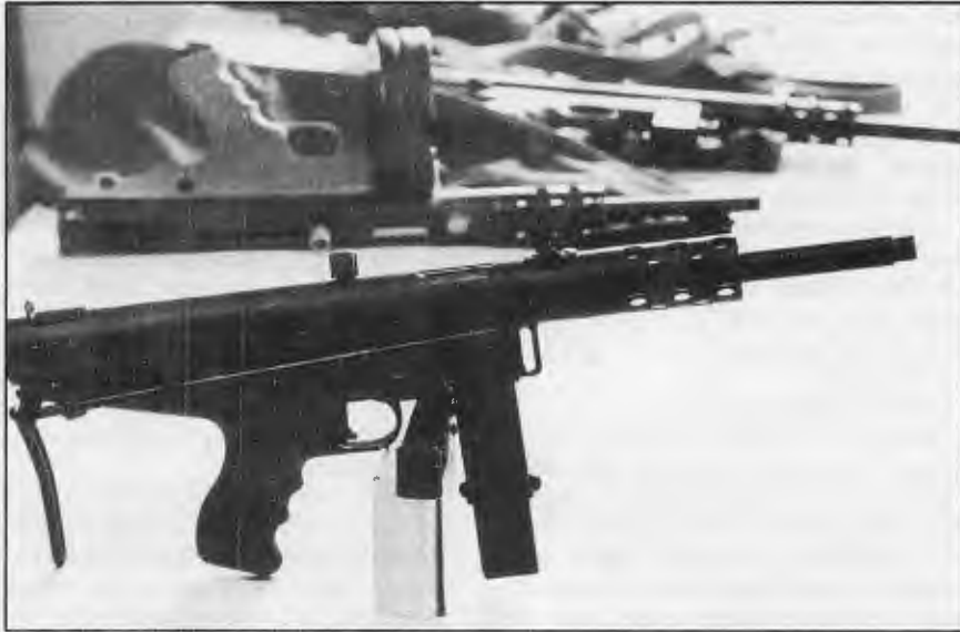
In background is drum magazine HS-91, with receiver made from square tube. The "Transformer"-toy cleverness of the basic design renders it adaptable to almost any available magazine or potentially changing available materials. Photo: Roman Majetic
