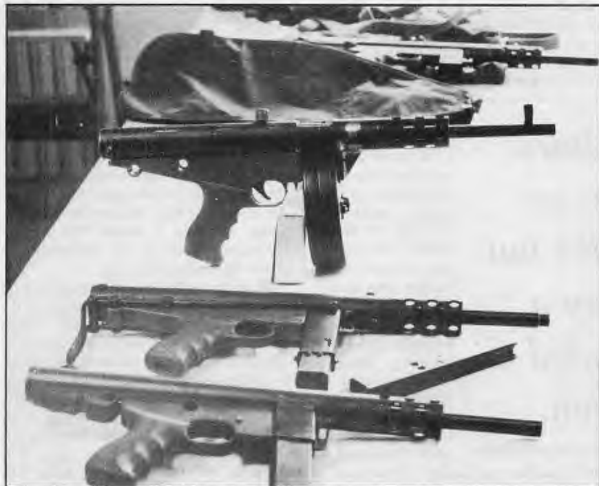
Tubular-receiver HS-91 submachine guns, showing how basic model is adapted to various available stick or drum magazines. In background is canvas bag that comes with weapon. Photo: Roman Majetic
