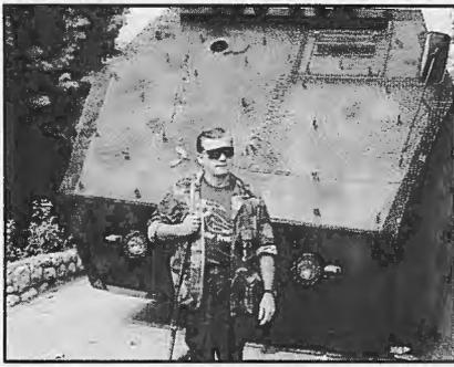
Turner in front of Croatian APC in Petrinja. Vehicle consists of steel plate, welded over flatbed cargo truck by Croatian metalsmiths. Photo: Jim Wallace
