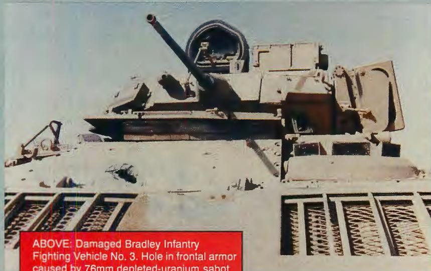
ABOVE: Damaged Bradley Infantry Fighting Vehicle No. 3. Hole in frontal armor caused by 76mm depleted-uranium sabot round; turret lifted from hull.
