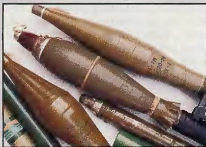
Top to bottom: product-improved PG-7 grenade with improved fuzing, ignition and motor performance; U.S. 81mm bomb mated to PG-7 rocket motor; OG-7 antipersonnel fragmentation round. Standard PG-7 grenade can be identified by fluted warhead; and PG-7 boosters of assorted ComBloc origin.
