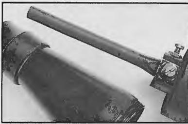
RPG-7V training device — barrel is exposed when dummy nose cone is unscrewed. Screws are turned in or out to adjust windage and elevation zero by bending the barrel one way or the other.
