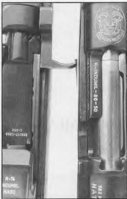
Markings on rare experimental M1 Garand and Model 52 bolt-action rifles indicate conversion from .30-06 to 7.62x51mm NATO. Note Colombian crest on receiver ring of Mauser.
